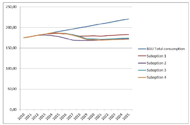
Power consumption of networked equipment in a condition of standby from 2010 until 2025.
